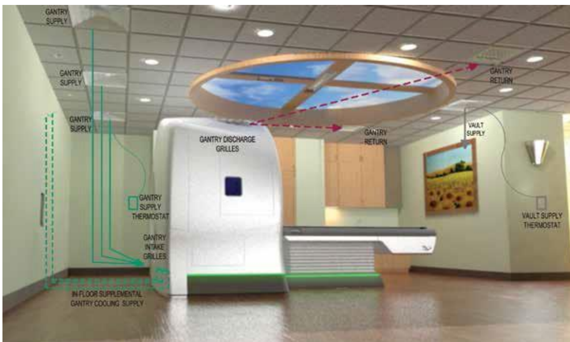
Figure 9 Radixact™ System Gantry HVAC Schematic
